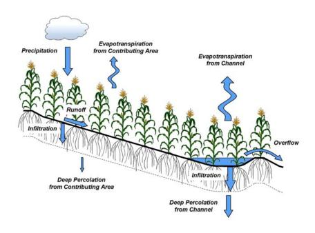
Figure 2. Water balance components of terraced land.
