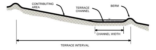
Figure 3. Cross Sectional View of Typical Terraced Land.
