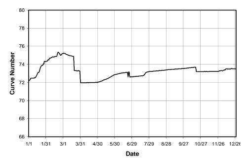
Figure 5. Simulated change in curve number due to tillage and erosion effects.
