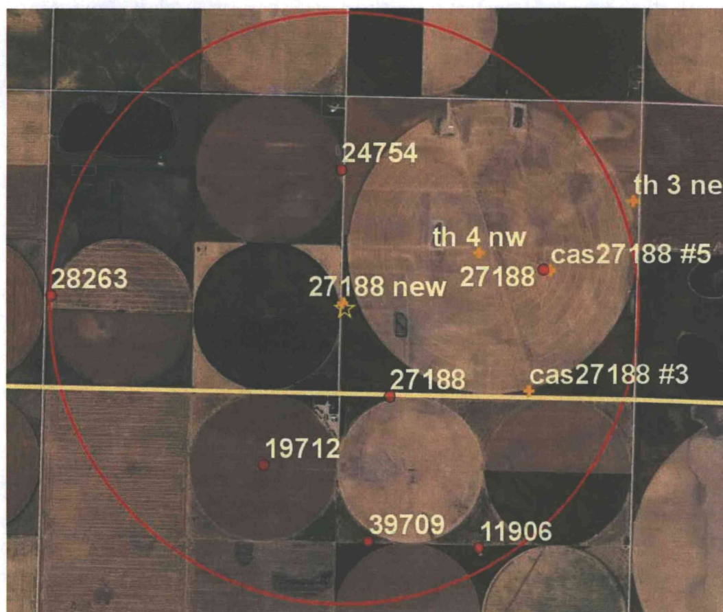
Figure 2 - New irrigation well 27,188 located in the center of the red one-mile circle. The star to lower right of the new well represents the observation well located 89 feet to the southeast. Farther to the lower right is the other irrigation well 27,188 operated in 2018. The five other irrigation wells operated and monitored in 2018 were 24,754 to the north, 28,263 to the west, 19,712 to the southwest, 39,709 to the south and 11,906 to the southeast. Water levels were monitored at the other four well casing locations to the east labeled "th 4 nw", "th 3 ne", "cas27188 #5", and "cas27188 #3". The Reiss domestic well located in the ne \frac{1}{4} , ne \frac{1}{4} , ne \frac{1}{4} of Section 15, Township 32 South, Range 31 West, is to the south of the new irrigation well 27,188 and is between irrigation wells 19,712 and 27,188.
