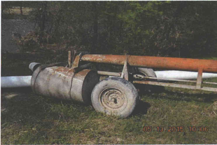
Diversion equipment on left bank at pumpsite
