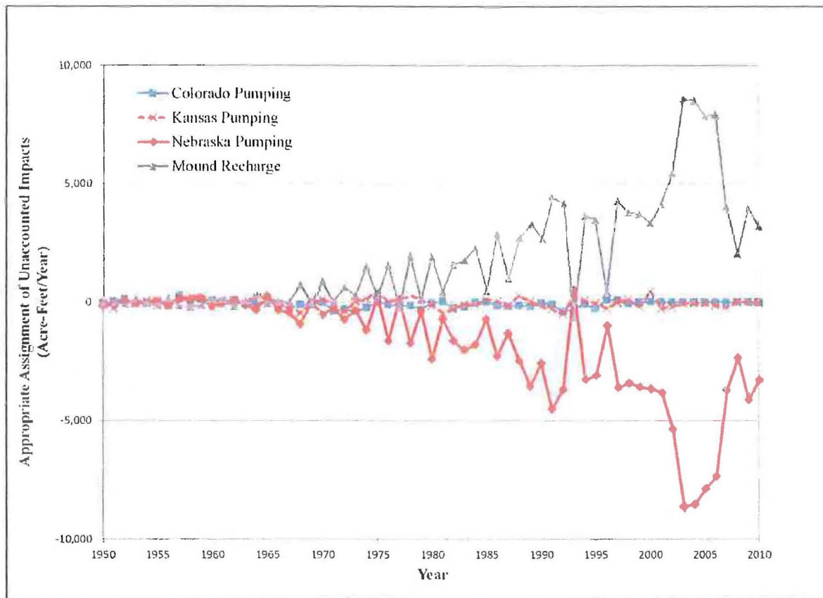
Figure 20. The Appropriate Assignment of Unaccounted Impacts for Colorado groundwater pumping, Kansas groundwater pumping, Nebraska groundwater pumping and mound recharge in the Swanson-Harlan Reach.
